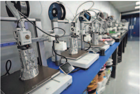
A 3D printing shop in the plant helps rapidly produce tools and parts.
